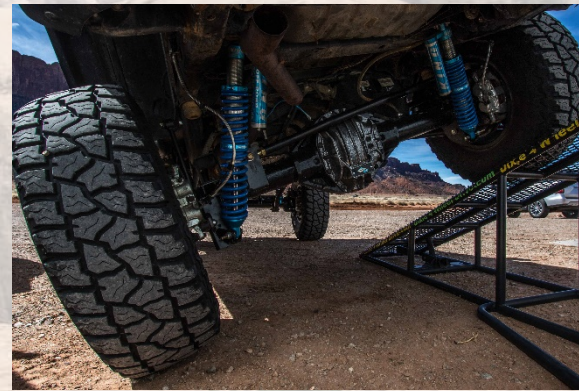
Jeep® Wrangler JK with Ultimate Dana 80™ rear axle and Ultimate Dana 60™ front axle
