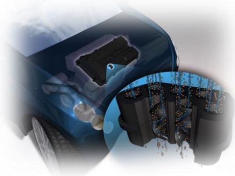
Adaptive Air/Oil Separator
