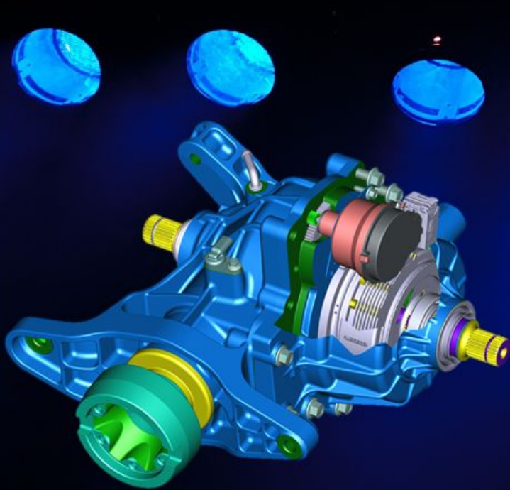
AdvanTek® Disconnecting All Wheel Drive Unit
